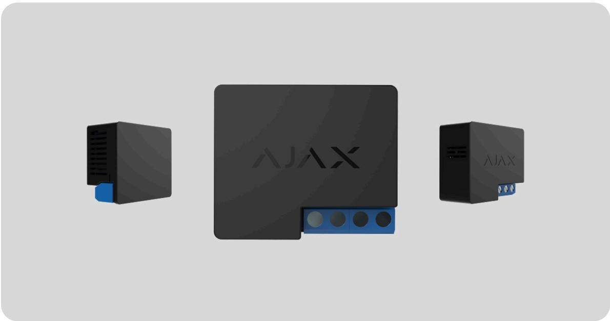
**WallSwitch** is a power relay to control 110/230 V~ power supply remotely. The relay power supply is not galvanically isolated with terminal blocks; therefore, WallSwitch switches only the power received at the power supply terminal blocks. The device has an energy consumption meter and features three types of protection: voltage, current, and temperature.
