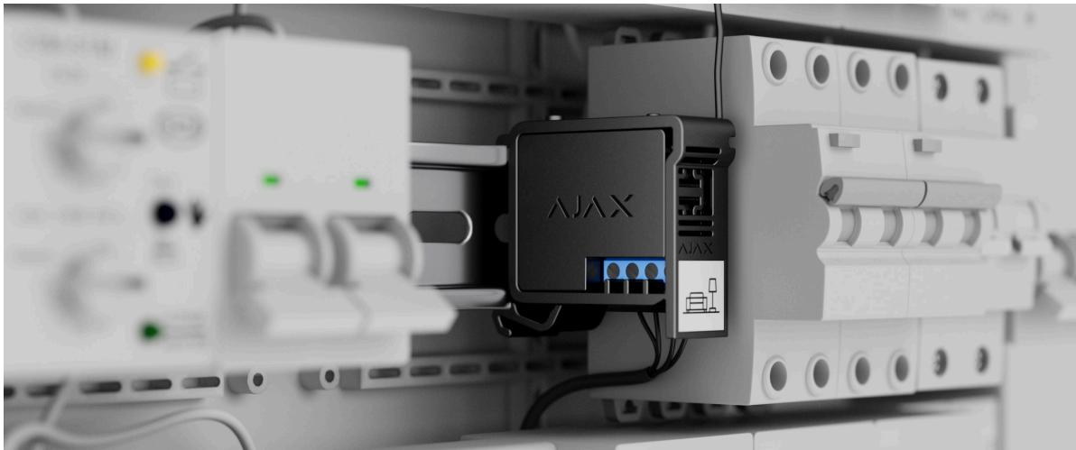
The device is connected to the 110/230 V~ grid. The WallSwitch dimensions (39 × 33 × 18 mm) allow installing the device into the deep junction box, inside the electrical appliance enclosure, or in the distribution board. A flexible external antenna ensures stable communication. To install WallSwitch on a DIN rail, we recommend using a [DIN Holder](#).
