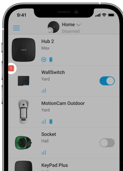
In case of a WallSwitch fault (e.g., no Jeweller signal between the hub and the relay), the Ajax app displays a malfunction counter in the upper-left corner of the device icon.
